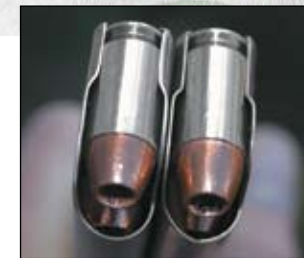
Cobramags offer unparalleled reliability partly through the use of a stainless body that has larger internal volume. One of the Cobramag's key features is a new follower design (below, l.) that integrates a stainless steel reinforcement at the front and left side where stresses are greatest. The magazine's feed lips (below, r.) grasp cartridges more firmly.
