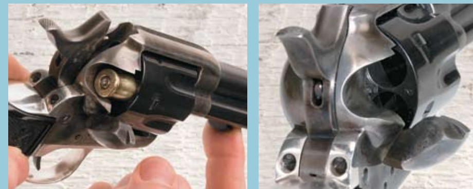
The Gunfighter is intended as an upgrade from a stock entry-level gun for competition. Internally, the revolver has a set of Wolff U.S.-made springs. Otherwise, the gun remains faithful to the original Model 1873 with its loading gate on the frame's right side.
