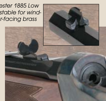
Pulling the lever down and forward drops the breechblock and allows the chamber to be loaded. Dual, spring-loaded detent balls (arrow) help keep the 1885's action closed.
